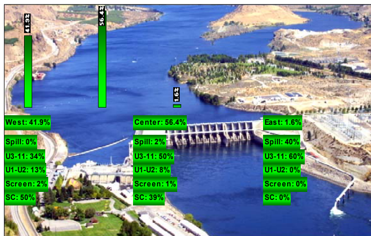
Figure 2. Proportion of sockeye across the river, directly upstream of Rocky Reach Dam at the Boat Restriction Zone, with the associated route specific passage at the dam in 2008. The proportions of detections have been grouped into three categories: west side, center or east side of the river.
